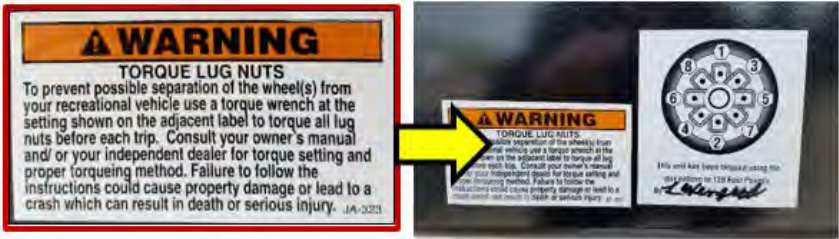
Lug nut torque pattern and warning label
