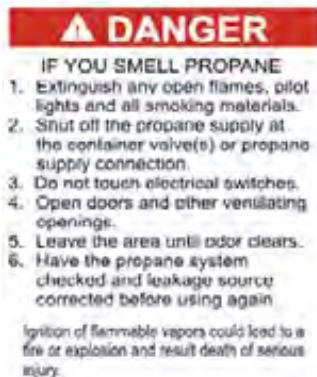
Propane System Label
