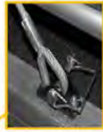
Safety Pin Cable hook-up on the cargo door
